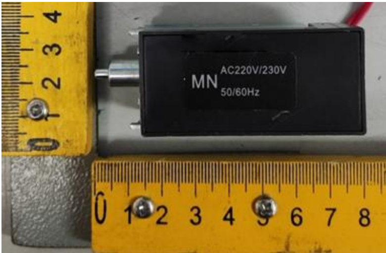
欠压脱扣器, Us: AC220/230V 50/60Hz
