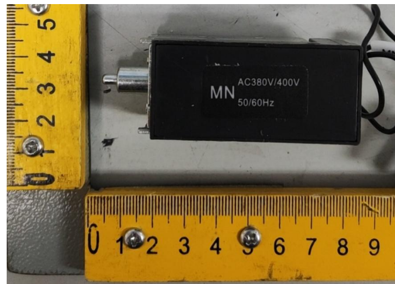
欠压脱扣器, Us: AC380/400V 50/60Hz
